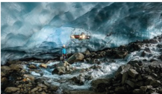
On the left, an englacial drainage conduit at the substrate contact of Gorner Glacier mapped with a LiDAR equipped collision-tolerant drone, On the right, an example of hyperspectral sound monitoring of an extreme flood in karstic conduits.
